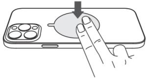
3. Paste the metal ring onto the center of the phone back by use of the alignment card
