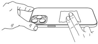
2. Paste the separation film onto the center of the phone back
