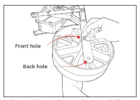
Align the center hole of Rear wheel (B) to the back hole of main body frame (D). Tighten nut to secure rear wheel (B).
