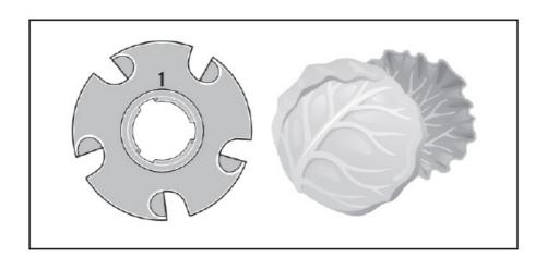
Insert the seed plate into the RC36 hopper by placing it over the center of the mounting and turning the plate clockwise to lock it into position.
