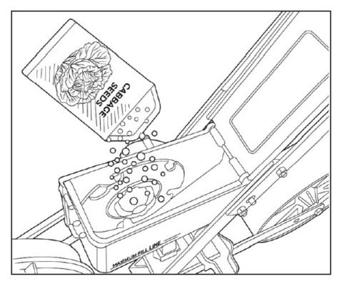
7. The SMITH® RC36 Single Row Seeder is now ready to use. It is always best to mark out a straight line before starting the first pass. An easy way to do this is to attach a piece of string to pegs at both ends of the planned row.
