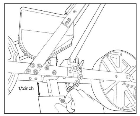
5. Adjust the row marker to the correct distance as shown.
