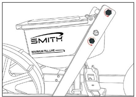
4. Align the holes of Handle Section (C) with the bolts protruding from main body frame (D). Place handle section (C) onto main body frame (D) and tighten the highlighted nuts.
