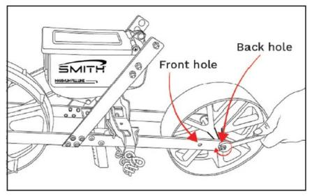
3. Remove the highlighted nuts from main body frame (D). Remove the same nuts on the reverse side.
