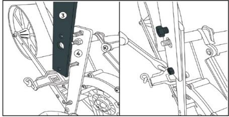
5. Take row marker arm (E) and remove the nut located at the bottom end.
