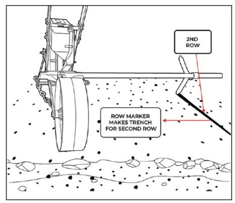
9. Stop at the end of the first run and place the marker back in its holder in the vertical position. The marker will have left a trail to be followed for the next seeding row (2nd Row). Now place the marker on the opposite side (on your left) and push the seeder along the track made by the marker on your first run (2nd Row).
