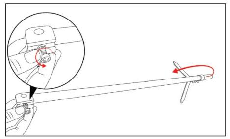
6. Place the bolt protruding from row marker (E) into the hole shown on main body frame (D). Secure row marker (E) with the nut you removed in step 5.
