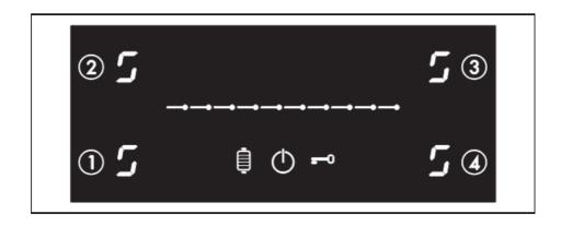
Press all the buttons of the cooking zones in sequence in a clockwise direction starting from the front left (1). A beep will sound to confirm every effective press of a button.
