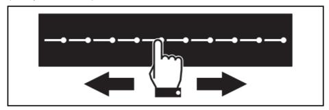
The display of the zone being used will indicate the selected power level. Intermediate power levels can be set:
