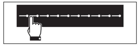
The display of the cooking zone used will turn on: the power level indicated is "1".
