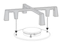
Make sure that the pan supports are ssimplified on their respective burners, without forcing them to be raised or tilted. If they are, repeat the positioning procedure. If you find that a pan is particularly unstable, make sure that the grids have not been positioned incorrectly.
