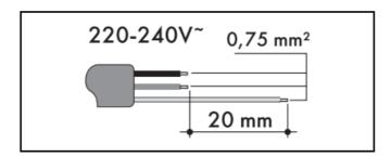
The values indicated refer to the cross-section of the internal conductor.
