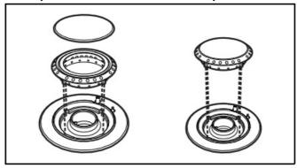
• Before lighting the hob burners, make sure that the flame-spreader crowns are correctly positioned in their housings with their respective burner caps.
