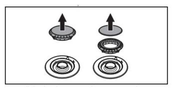
3. Pull the knobs upwards to remove them.
