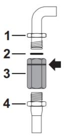
• Apply insulating material to the thread of the gas hose connector 4 and screw the adapter 3 onto it. Screw the assembly onto the movable connector 1 of the appliance, inserting the seal provided 2 between them.
