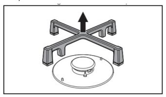
2. Remove the flame-spreader crowns and relative burner caps.
