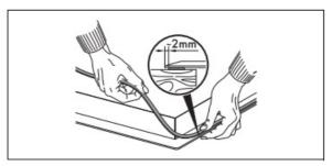
• Do not use silicone to secure the hob. This would make it impossible to remove the hob without damaging it.
