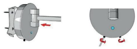
Tighten screws and retighten later if needed.
