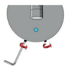
Tighten screws and retighten later if needed.
