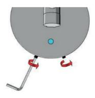
Tighten screws and retighten later if needed.
