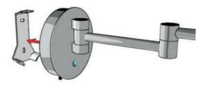
Drill a hole of Ø50 mm and 15 mm dept to the wall.
