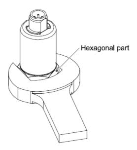
•When piping, apply a spanner to the piping section of the sensor.
