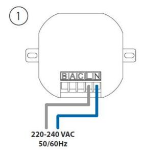
• Connect the phase wire (brown) to L and connect the neutral wire (blue) to N.
