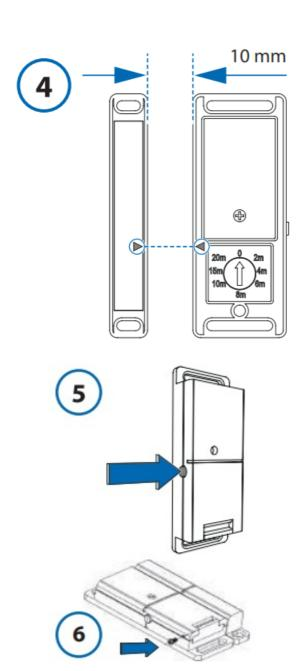
• **B.** Set the switch-off time to the preferred position by rotating the rotary switch between 0 and 20 min (2). 2-20 min: After the set time has expired, the receiver will automatically switch off.
