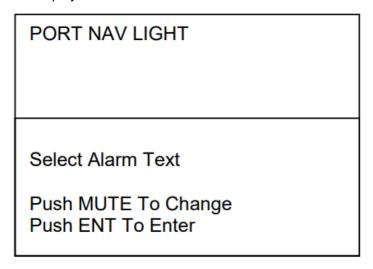
Use the Select Up or Down key to scroll through the pre-named Alarms. Once you have found the one required press the ENT key.
