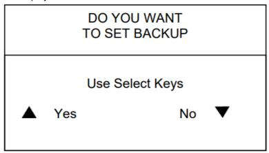
If Yes is selected the second NV-100 I/O Box (Rotary Switch Position 3) will copy the primary I/O Box and the system will then return you to the Set-Up Menu.
