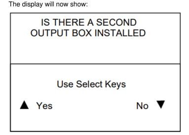
If Yes is selected the system will continue on from Output 8 to Output 9, etc. If No is selected the system will
