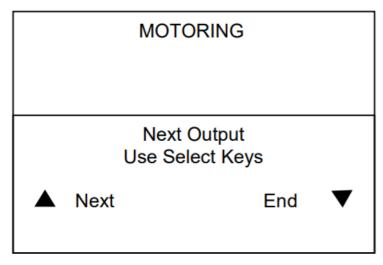
Press the Select Up key to set the next Output for the group or if this is the last, or only, light being associated to the group, then press the Select Down key to exit. If End is selected the system will return to the Set-Up Menu.
