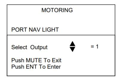
Use the Select keys to select the Output you want to join to the Group, once you have scrolled to the Output you want to join to the Group press the ENT key.
