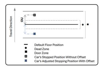
Offset Up [OU] = Car Position After Stopping – Default Floor Position [units in mm] ◆ Configuration:
