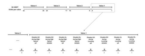
Step 1: Replace 0 with 1 to disable the required valve commands for valve 1
