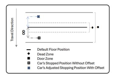
Offset Down [OD] = Default Floor Position – Car Position After Stopping [units in mm] ◆ Configuration:
