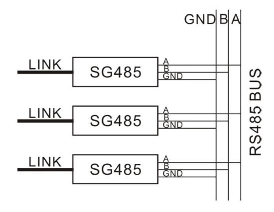
Please set each controller's communication address before networking and same module address within the same network is not allowed.
