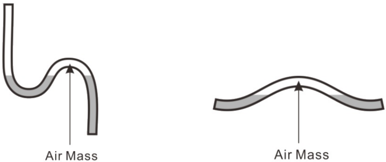
Fig. 3 – Incorrect Pipe Connection Methods
