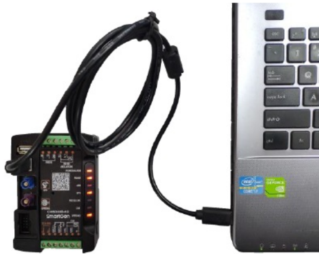
Fig.8 – USB and PC Device Connection Diagram
