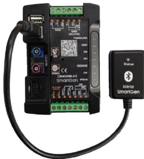
Fig.9 – USB and SGB100 Module Connection Diagram
