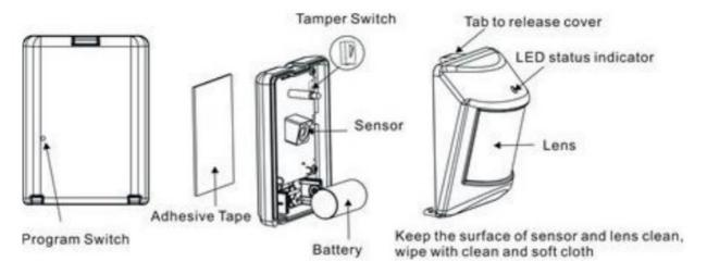
Nota: Inclusion button is located on the back cover and you can press it through the use of a spike.
