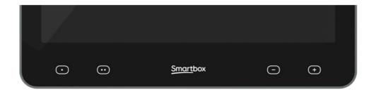
Buttons 1, 2 and the Smartbox button can help you control and navigate your Grid Pad device when using Grid, or they can be customised using Grid's set of powerful commands. You can customise the colour of the smart button highlight as well as add audio feedback. The two Smart volume buttons cannot be customised and offer eye access when using Grid.
