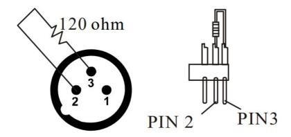
If you wish to connect DMX-controllers with other XLR-outputs, you need to use adapter cables. The transform of the controller line of 3 pins and 5 pins (plug and socket)
