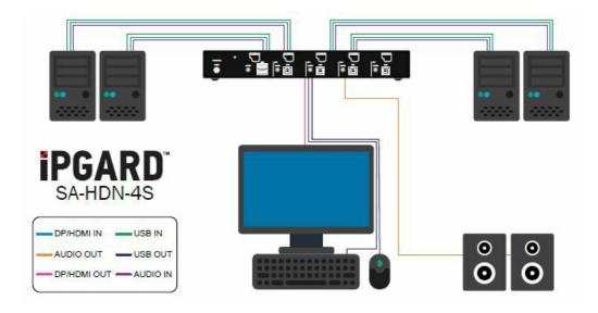
A full Manual can be downloaded from <a href="www.ipgard.com/documentation/">www.ipgard.com/documentation/</a> Advanced 4-Port Secure Single-head DP/HDMI to DP/HDMI KVM Switch with Audio Quick Start Guide
