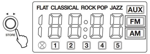
For 1st time use, the default is 87.5/FM or 526.5/AM, frequency modulation can be adjustable by rotating button 5.
