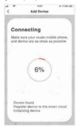
6. In the automatic network connection Mode, the indicator flashes quickly, holds the reset key for 5 seconds with the card pickup pin , the indicator flashes slowly, and enters the manual network connection mode. APP chooses compatible mode. According to the prompt, enter'WiFi password "and click confirmation , then switch to the WIFI settings interface. Connect Smartlife-XXXX network and return to APP to continue adding devices.
