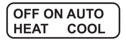
The lower left corner of the display controls the mode selection, depending on how your installer has set your SMT-710 up you will be given the option of selecting On and Off with a single set point (with a preset differential between the heating and cooling) or selecting individual heating and cooling modes, each with individual heating and cooling set points.
