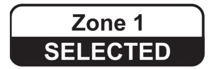
its ability to manage two independent zones. These zones are identified as either Zone 1 (The location of the wall Controller) and Zone 2. If the zone is shown as "selected" then conditioned air will be sent to this area and the air conditioning will turn on and off to maintain this zones temperature.
