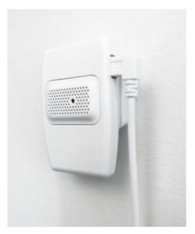
3. Insert the power cord into the sensor.
