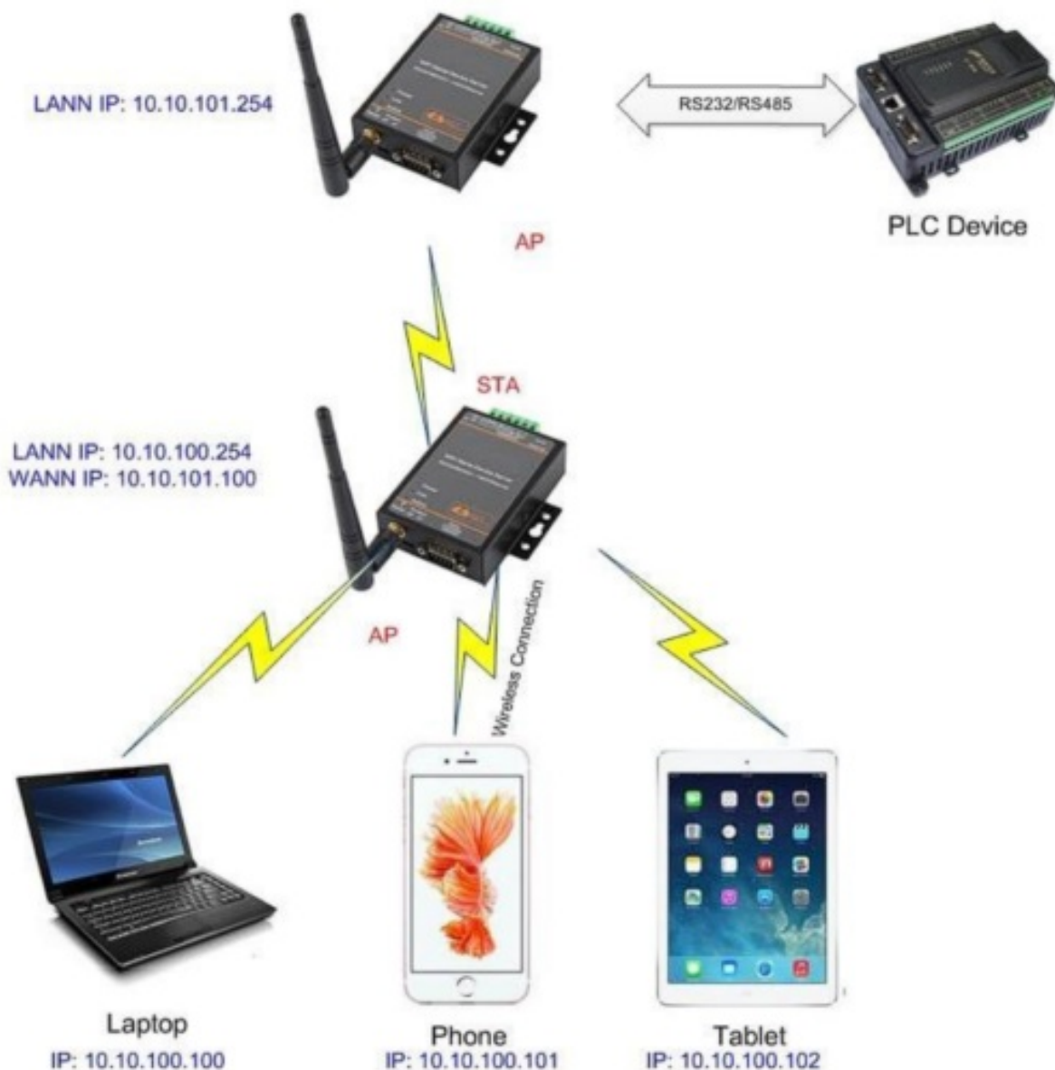
Figure 14. AP+STA Wireless Network
