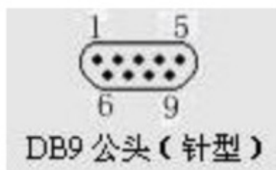
Figure 4. RS232 Pin Definition (Male/Needle Type)
