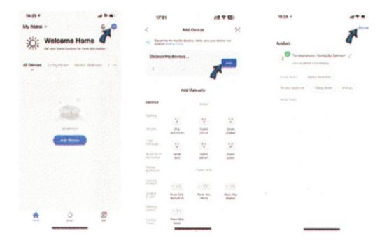
After connecting to WiFi successfully, click the sensor icon to enter the app interface and do the settings. You can preset the value of temperature and humidity for alarming from here.
