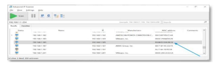
Note the IP address of the gateway. You need this to install the gateway. link it to your home automation package.
