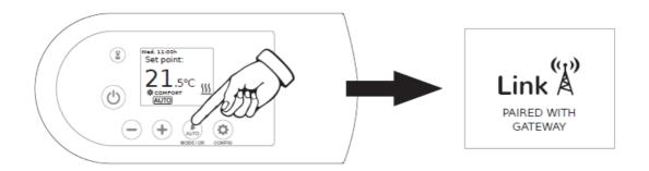
To pair the Energy Monitor press using the clip supplied, the small push button on the top of the Energy Monitor. Refer to the Status of the Energy Monitor LED chart (Below) to check that it is paired. Your Energy Monitor is now connected to the Gateway.
