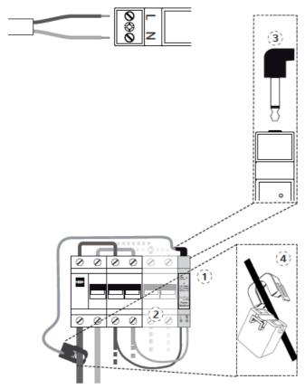
Place the Energy Monitor in the DIN rail on your control panel where there is available space. 1 Connect the other two ends of the cable to the output of a circuit breaker switch, preferably a lighting type, minimum 5A/230V, 2 The said circuit breaker must be arranged so that it is easy to access and it must be marked so that it can be recognized as the equipment disconnection device.
