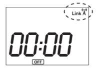
To pair the towel rail press the OK button for 5 seconds until the icon appears in the top right of the screen. Your Colorado DGi+ is now connected to the Gateway.
