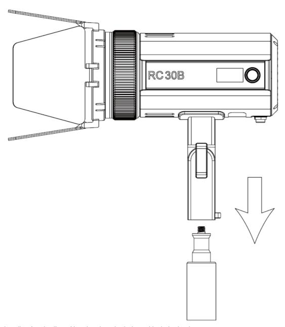
3. Insert the handle of umbrella softbox into into the hole and lock the knob.
