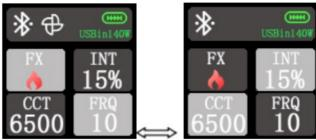
Rotating the INT/ FX knob clockwise/ counter-clockwise at this point adjusts the 9 x light effects/ brightness ratio corresponding to the cursor area.
