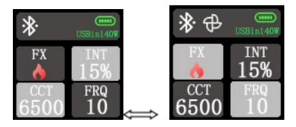
In FX mode, rotating the knob clockwise/ counter-clockwise adjusts the color temperature/ frequency corresponding to the cursor area.
