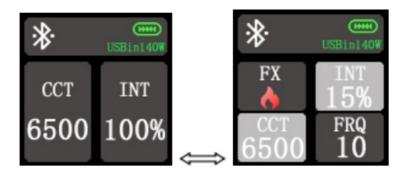
In CCT/ FX mode, long-press the mode button 2s to store the current parameters and goes into the PRESET mode. Rotate the INT knob to select the presets and click to confirm. Long-press the button 2s again or select the preset to exit. Up to four sets of preset parameters can be stored. The screen display will change as follows.
