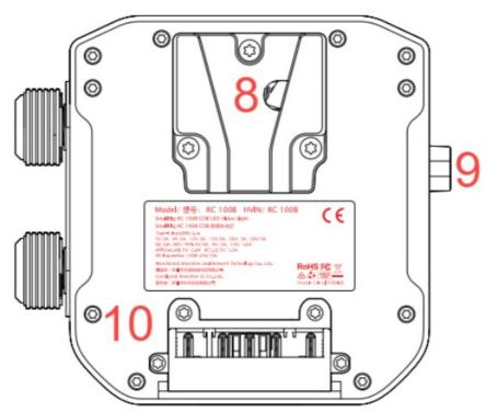
**BP Input Interface:** You can provide a mobile power supply solution for the RC 100B through the V-Mount battery or NP-F battery plate. It supports 100W V-Mount battery input/60W NP-F battery input.
