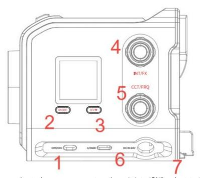
ON/ OFF Switch: After connecting to the power source, turn the switch to "ON" and rotate the INT knob one round to power on the RC 100B; turn the switch to "OFF" to shut down. The Bluetooth name suffix of the gear will be displayed at the bottom of the white startup interface. The screen display will change as follows.
