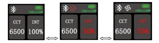
After powering on, long-press the Bluetooth/ Mute control button to reset the Bluetooth connection. The Bluetooth icon will flash quickly. You can open the SmallGoGo application and set up a network for the gear based on the Bluetooth suffix prompted during startup. If you haven't downloaded SmallGoGo before, please scan the QR code below for more information and download, or search and download it from app stores such as Google Play/App Store.
