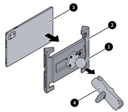
3. Step 3: Install the ball joint 2 of the base into the other ball socket of the adapter bracket 1, and rotate the handle clockwise to firmly fix the terminal.
