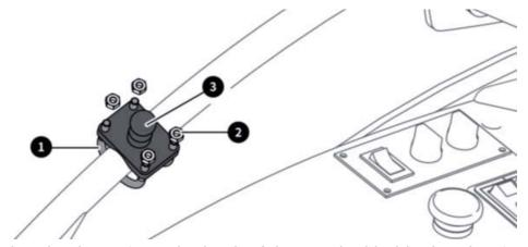
2. Step 2: Fix the bracket base 1 on the back of the terminal holder bracket 2 with screws and place in and fix the terminal 3. Rotate the handle of the adapter bracket4 counterclockwise to loosen the ball socket, and then install the ball joint on the back of the terminal into the ball socket of the bracket.
