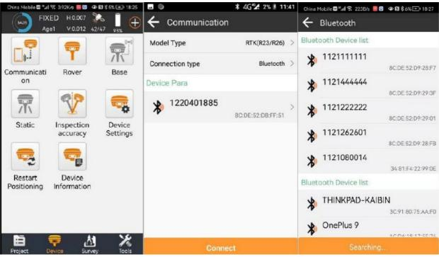
2.2 Set R26 base as base (after the setting is completed, please wait 2 to 3 minutes before clicking Stop to disconnect, then connect another R26 and set it as rover. Because it takes some time to update the device information): Device -> Base -> Set base station startup parameters -> Set Base Startup,
