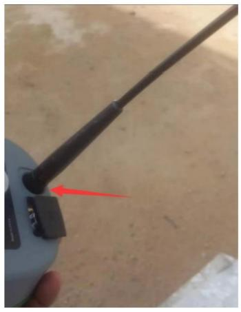
1.3 R26 needs to work in an open and unobstructed place to ensure accuracy
