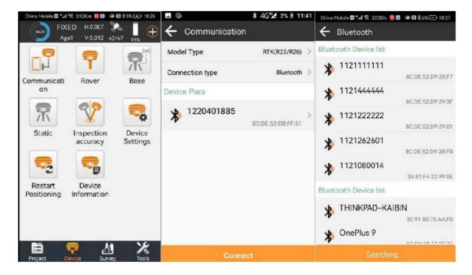
3.2 Set R26 rover as rover Device -> Rover -> Set rover startup parameters -> Set Rover Startup, Please note that if you use radio RTK for correction, the radio protocol and frequency when you set up the rover must be the same as your base. If you want to use another brand of radio base station, please pay attention to whether it supports the R26 radio protocol and frequency.
