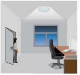
With sufficient natural light, the With insufficient natural light, the sensor switches on the light automatically when presence is detected.
