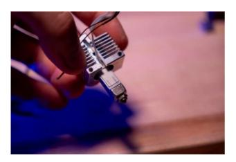
Step 4: Slide the retaining clip onto the bottom of the heater to hold it in place while you complete the next step.
