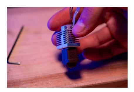
Step 8: Now screw your fan into the heatsink with a 2 mm hex key.
