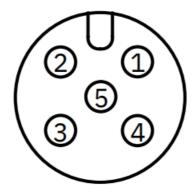
Pin 1 NC Pin 2 NC Pin 3 GND Pin 4 CAN-H Pin 5 CAN-L
