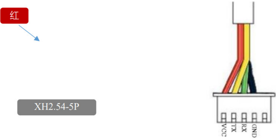
Figure 3-1 RPLIDAR S3 Pins
