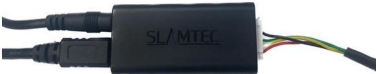
Figure 2-2 Connect the USB Adapter to PC via Micro-USB Cable
