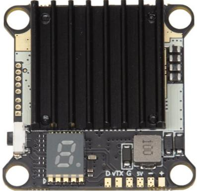
The TX2501 is powerful VTX which have 2.5W output, the heat sink dispatch the heat quickly from VTX, LED segment make the VTX easy to set and check the BAND/CH/POWER, its also support X Band(5G Hz) and Low Band.
