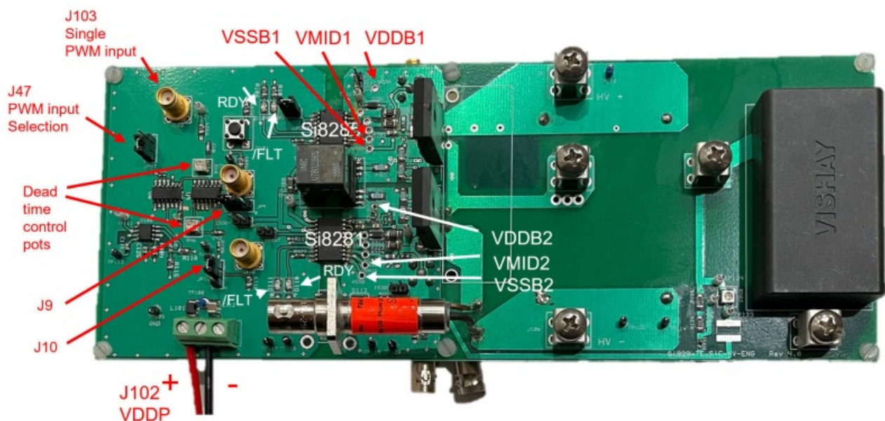
Figure 2.1. Si828x-HB-EVB Input Power and Input Signals
