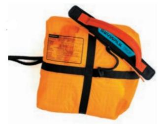
2. Now you can connect the V-lines of the DROP with the lanyard of your reserve chute. To connect the reserve chute to the V-line, you must use a screw shackle with at least 2400 daN strength The lines have to be connected on both sides of the screw shackle and must be secured with rubber bands (option A). As an alternative, you can use a loop to connect the two lines together (option B).
