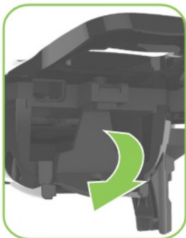
Open the battery latch (Press back of latch and flip down)
