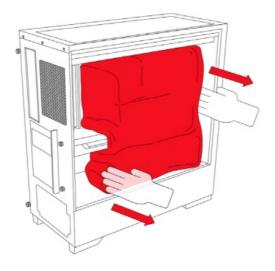
Note: Removing protective foam may disconnect cables. Refer to the next step
