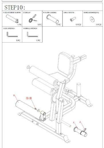
**Warning!** After installing the dumbbell, it is necessary to use the Weight Holder Clip to secure the dumbbell.
