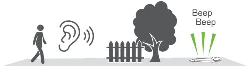
Audio tracer can be toggled on and off with stunt button when plane is not flying.
