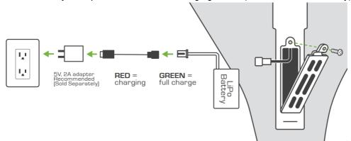
Once charged, disconnect battery from cable and reattach to plane. Tuck back into plane and secure door with screw. Remote will beep 1x every couple seconds when LiPo battery runs low.
