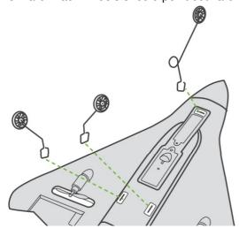
**INSPECTING AND REPLACING DAMAGED PROPS**
