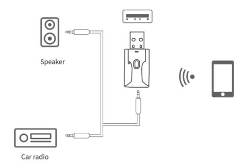
**Tips:** USB wireless adapter power consumption is low, when using mobile power supply, some will automatically turn off the power, priority is to use USB charger power supply, some TV USB port power supply is insufficient, will cause the adapter can not work properly.
