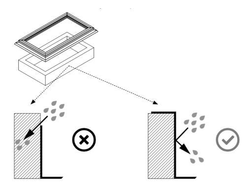
If the existing curb does not meet the above requirements, this may lead to functional issues including glass breakage, stress cracks, leaks, and visual imperfections.
