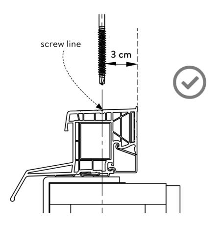
Guideline (\*): First screw at  $\pm$  60 mm from the side of the upper surface. Spacing no more than 40 cm.
