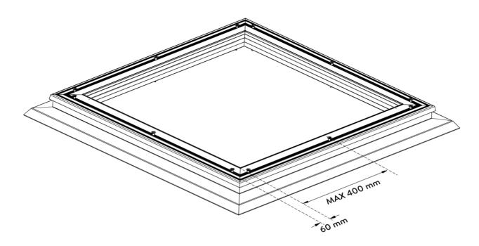
(\*) If the situation calls for it, don't hesitate to use additional screws. When combined with opening systems, additional screws should be used, with a maximum spacing of 200 mm.
