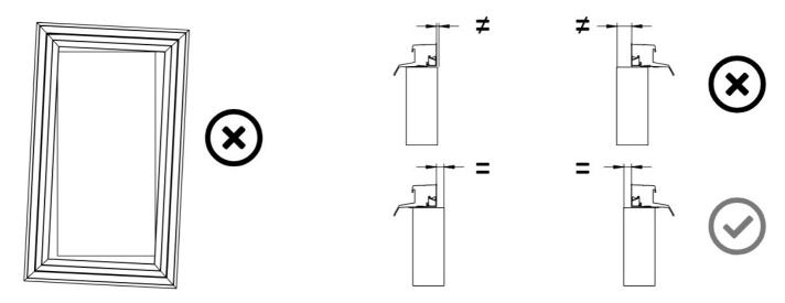
Make sure that the adapter frame is properly centred in relation to the curb!
