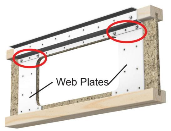
3. Install the lower Steel Flange. Place the lower Flange over the lower end of the Web Plates. Install two fasteners at each end of the Lower Flange through the lower ends of the Web Plates. Leave the fasteners loose enough to allow a small amount of play.
