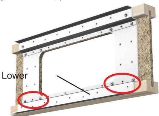
4. Install a fastener at each end of the lower Steel Flange. Leave the fasteners loose enough to allow a small amount of play.
