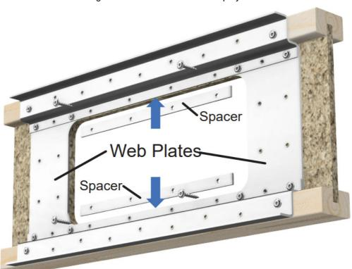
6. Tighten all initially installed fasteners. Pre-drill and install remaining fasteners.
