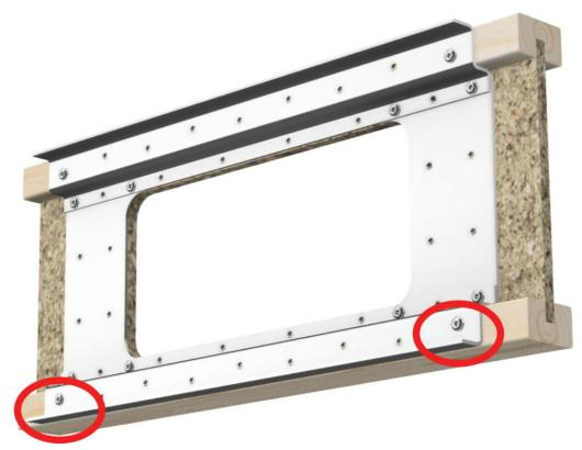
5. Place a the steel Spacers between the Web Plates and behind the steel Flanges. Install a fastener at each end. Leave the fasteners loose enough to allow a small amount of play.
