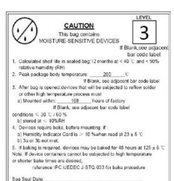
The module Must go through 125°C baking for at least 9 hours before SMT AND IR reflow process!
