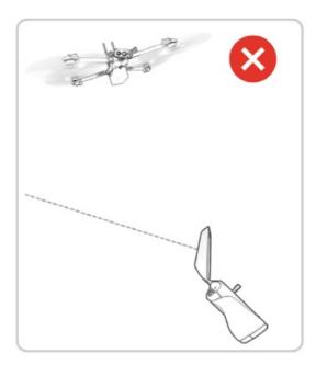
**WARNING:** The controller antenna is located in the cover and should be oriented in the direction of the drone to maximize RF signal quality.
