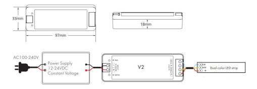
**Note:** Continuously switch off and on the power supply two times rapidly, It will change 3 levels color temperature (WW, NW and CW) in sequence.
