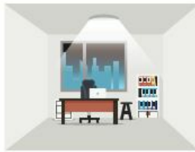
2. With insufficient ambient light, the sensor turns on the light when motion is detected.
