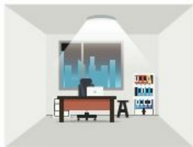
1. The sensor turns on the light and dim up to expected brightness level when motion is detected.
