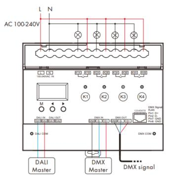
**Note:** The maximum surge current of the AC output is120A, the sum of surge current of multiple resistivel load or inductive load (LED drivers )should not exceed its maximum value. Otherwise, the product will be overloaded and damaged.
