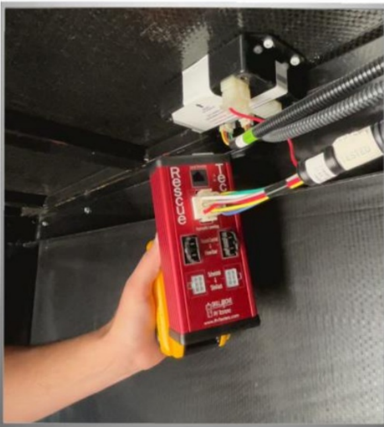
4. Select Hydraulic Leveling then select which jacks and what direction they need to move
